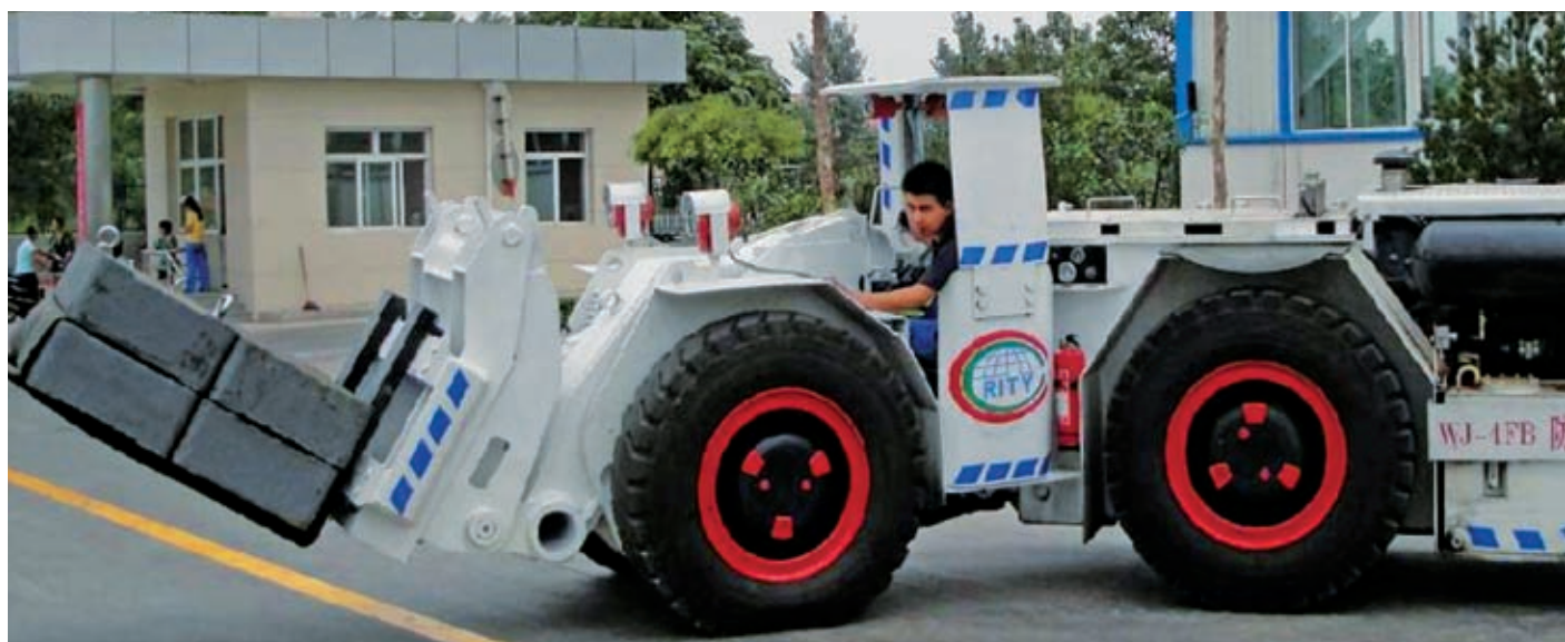
The WJ-4FB explosion-proof diesel oil scraper jointly researched and manufactured by Shengdong Coal Group and its suppliers.
