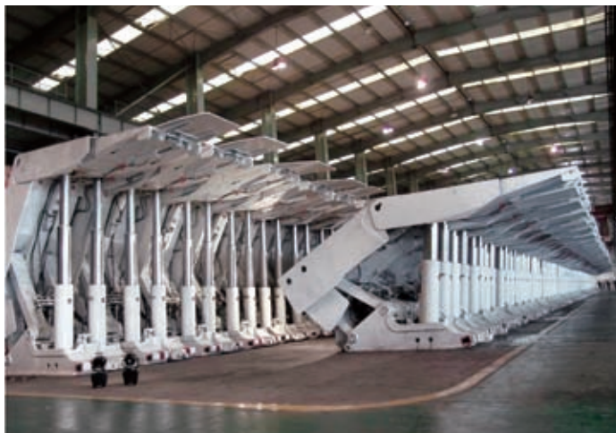
The domestically manufactured hydraulic supporter jointly R&D and operated by Shendong Coal and its Suppliers
